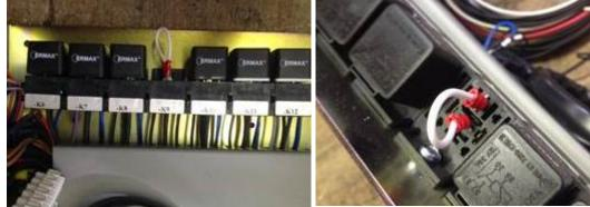
Relay – K9, is activating the shutdown, if the engine is overheating or is missing oil pressure.
