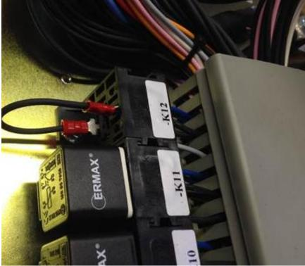
Relay -K12, is activating the shutdown, if the compressors is overheating.
