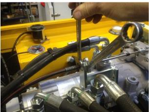
After the adjustment of the cable, it might be necessary to adjust the reverse alarm sensor.
