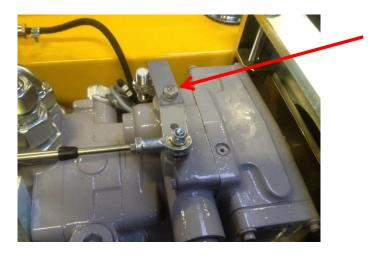
The cable can also be adjusted simply by moving the handle. This adjustment is not very accurate but easier. Move it just one "click" at a time.
