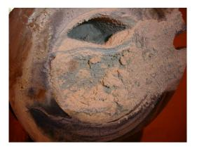
3. The screw pump shaft can be worn out due to much work or much work with very abrasive paint.
