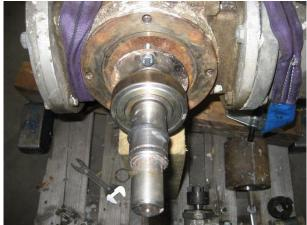
2) Mount the Circlip.
