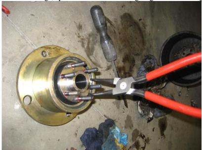
Mount the Bearing house. Remember Lock-tite and grease.
