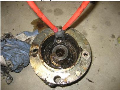
9 Disassemble the bearing house.
