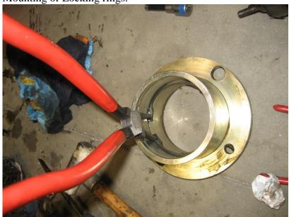
Mount bearings, spline hub and the locking rings in the housing.
