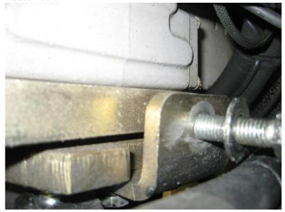
2 Loosen og remove 6 pcs. M8 nut and remove the pulley.
