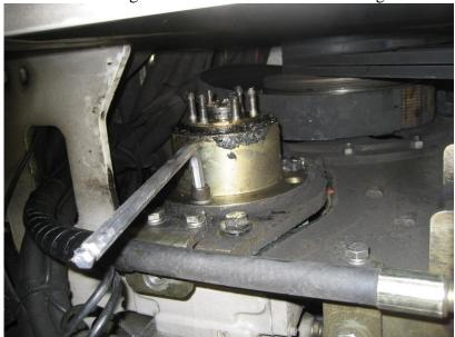
Mount the pulley onto the support and mount the belt.
