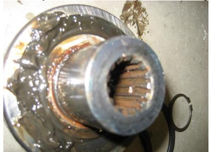
New Bearing, Spline hub and treading supports.
