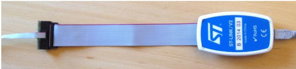
The small 10 pin plug, must be connected to X11 on the IO board of the LineMaster. It must be connected so the red "wire" is down.
