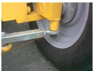
Here you adjust toe-in. Borum Standard toe-in is 0-2 mm measured on the rim
