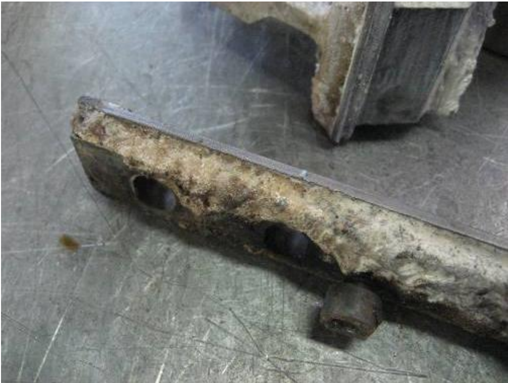
Clearance between dampers approx 0,2mm
