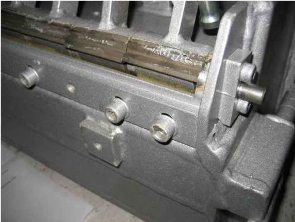
Clearance between dampers approx 0,2mm
