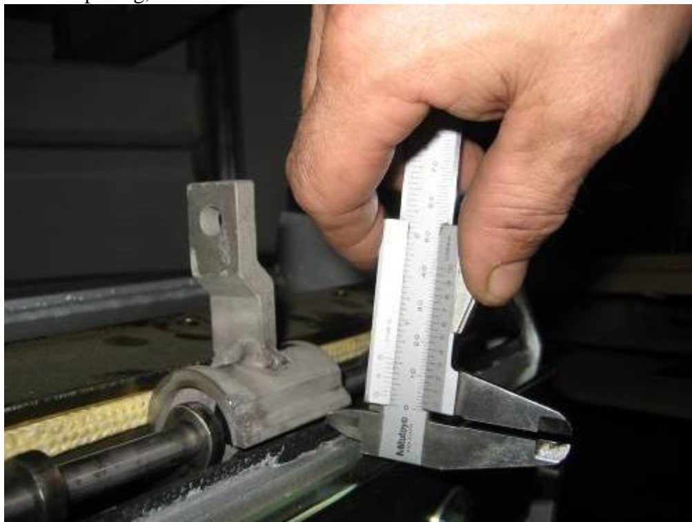
Shutter opening, 70-90 % of line thickness
